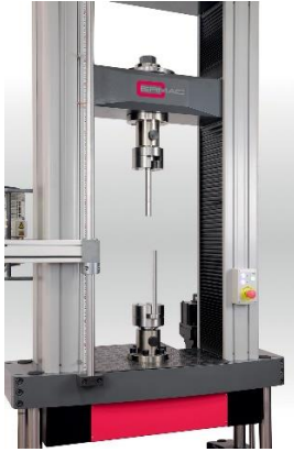
Fixtures for threaded specimens
