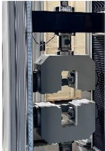
Hydraulically operated horizontal gripping system
